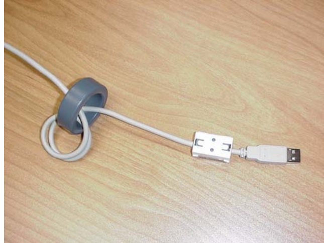
Figure 8 - Example of a USB Cable Using Ferrites
